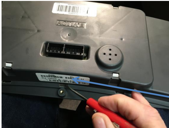
Pic 1. Push in and down on the 10 clear tabs starting in the middle as shown to release the lens.
