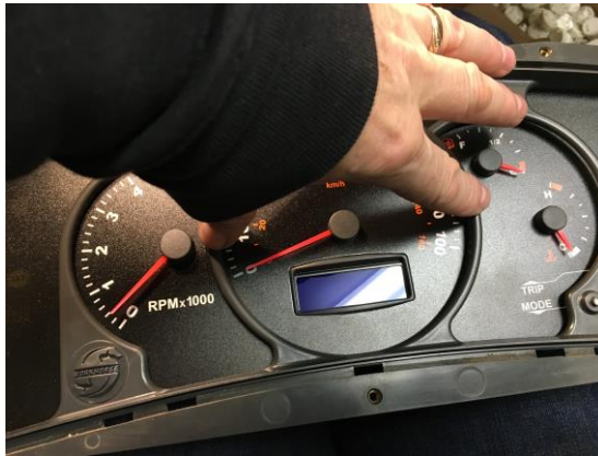
Pic 33. Press the trim back into place. If you have the brown mode and trip pins, you will need to make sure they are in place before you put the trim on.
