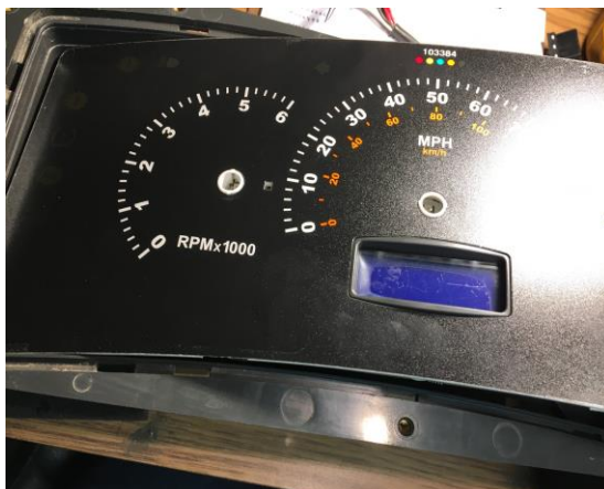
Pic 28. Position the face and circuit board into the housing and press down until the 4 white tabs lock into place.
