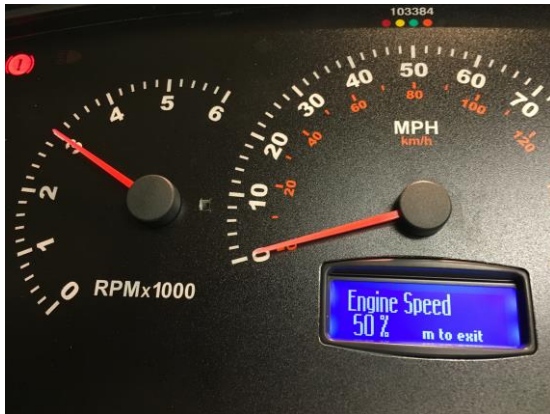
Pic 39. View of “Engine Speed” at 50%
