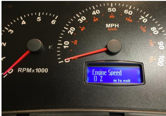
Pic 38. It will begin a sweep of each gauge, if adjustment is needed you will have to unplug the cluster and move the needle as needed. Always move the needle for RPM and MPH counter clockwise, and Fuel and Temp clockwise.
