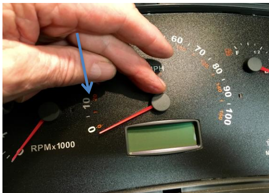
Pic 4. Lightly move to the park position of each gauge and make note of where they are pointing. You will need this info for when you put it back together.
