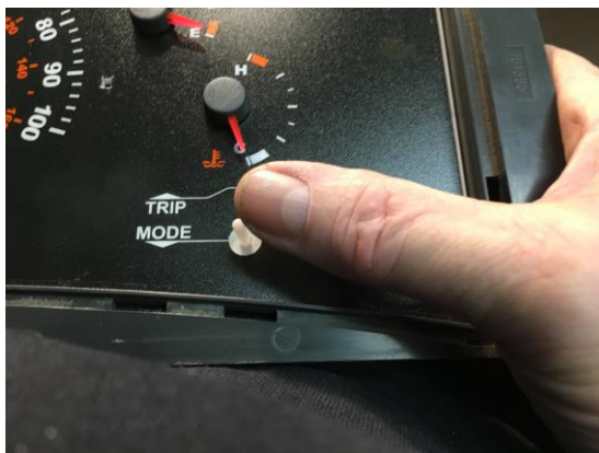
Pic 35. Do not install the cluster at this time; just plug it into the harness. For testing the needle position turn the key on and push the “mode” button in for 10 seconds.
