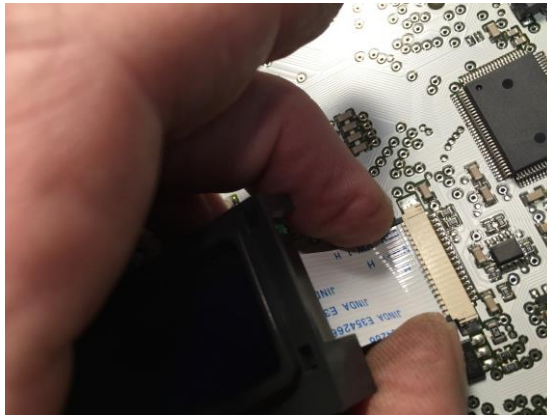
Pic 23. Push the black lock tabs in until it is seated against the socket.
