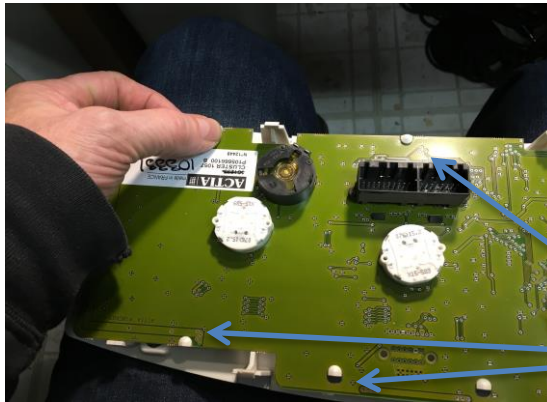
Pic 9. Push the 7 white tabs outward from the circuit board to release the circuit board from the face.
