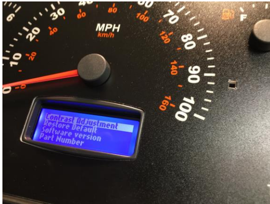
Pic 41. Should you want the contrast lighter or darker you can do this at any time by entering the diagnostic menu pushing the “Mode” button for ten seconds and scrolling to “Contrast”
