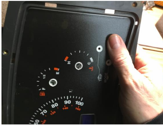
Pic 29. Push in on the face until it snaps into place.
