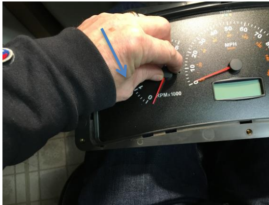
Pic 5. Twist and pull up needle by the cap in the direction that the gauge parks. Twist RPM and Speedo “counter-clockwise”. (Example 1)
