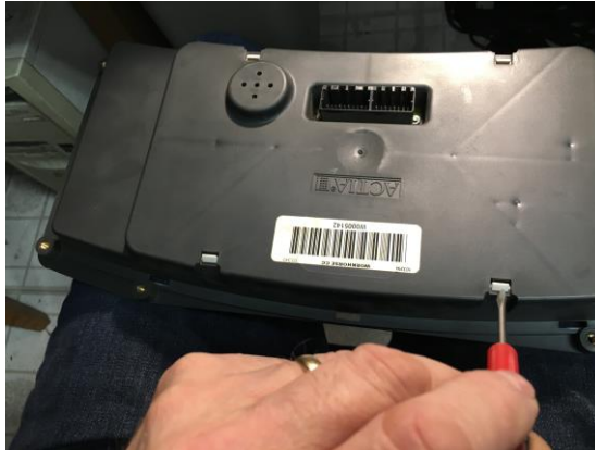
Pic 7. Push in and down to release the white face tabs. There are 4 of them.
