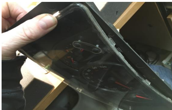
Pic 34. If you want to test your cluster in the vehicle before you put the lens on, save this step for last. When putting the lens back on start at the narrow ends first, snap those into place and then go to the mid point on the wide ends and snap those in and work your way around until it is fully seated.
