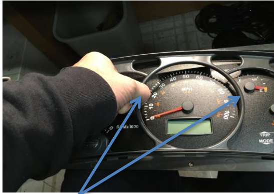
Pic 3. Remove the trim; there are 2 retainers at the 3 o'clock and 9 o'clock position. Press in toward the center of the speedo ring and pull up.
