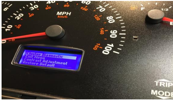
Pic 36. Scroll to “Cluster Diagnostics”... “Trip” scrolls up the menu and “Mode” scrolls down. By setting on a highlighted selection it will enter after about 2 seconds.
