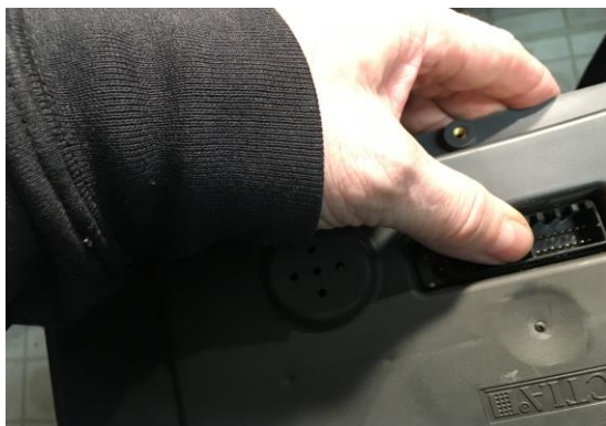
Pic 8. Push in the cluster connector to remove the face and circuit board.
