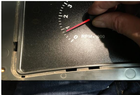
Pic 30. Install the needles by pushing on to the pins and twisting toward their respective park positions. You will want to point them exactly where they were when you took note step #4. Keep the cap of the needle about a fingernail width from the face so it won't drag on it.
