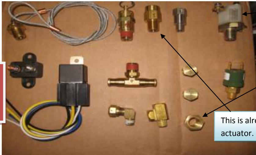
Always use thread sealant with any of the brass fittings or any fittings with pipe thread. DO NOT OVER TIGHTEN FITTINGS!
