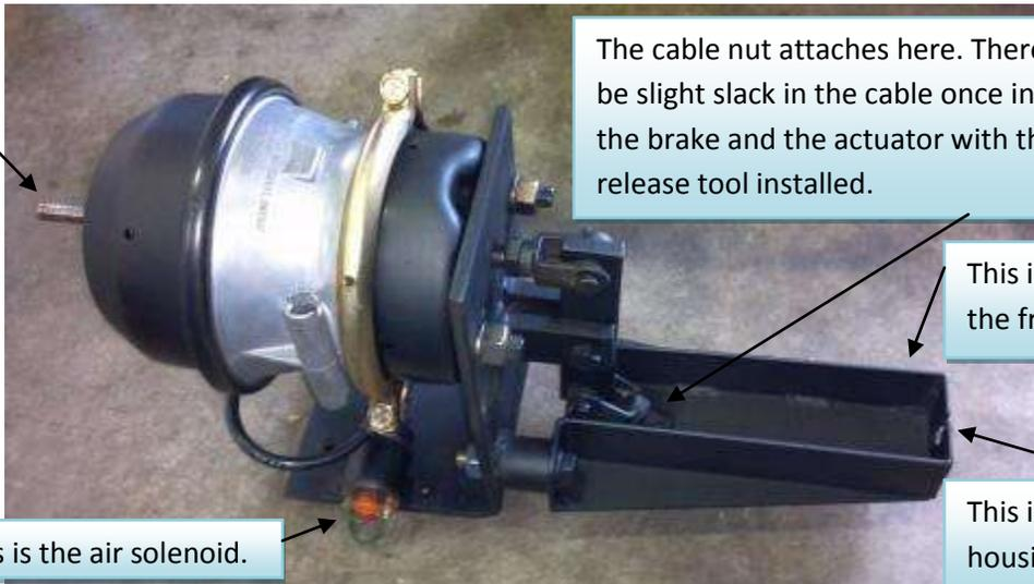
This is the release tool. With the nut all the way tight the brake is released.
